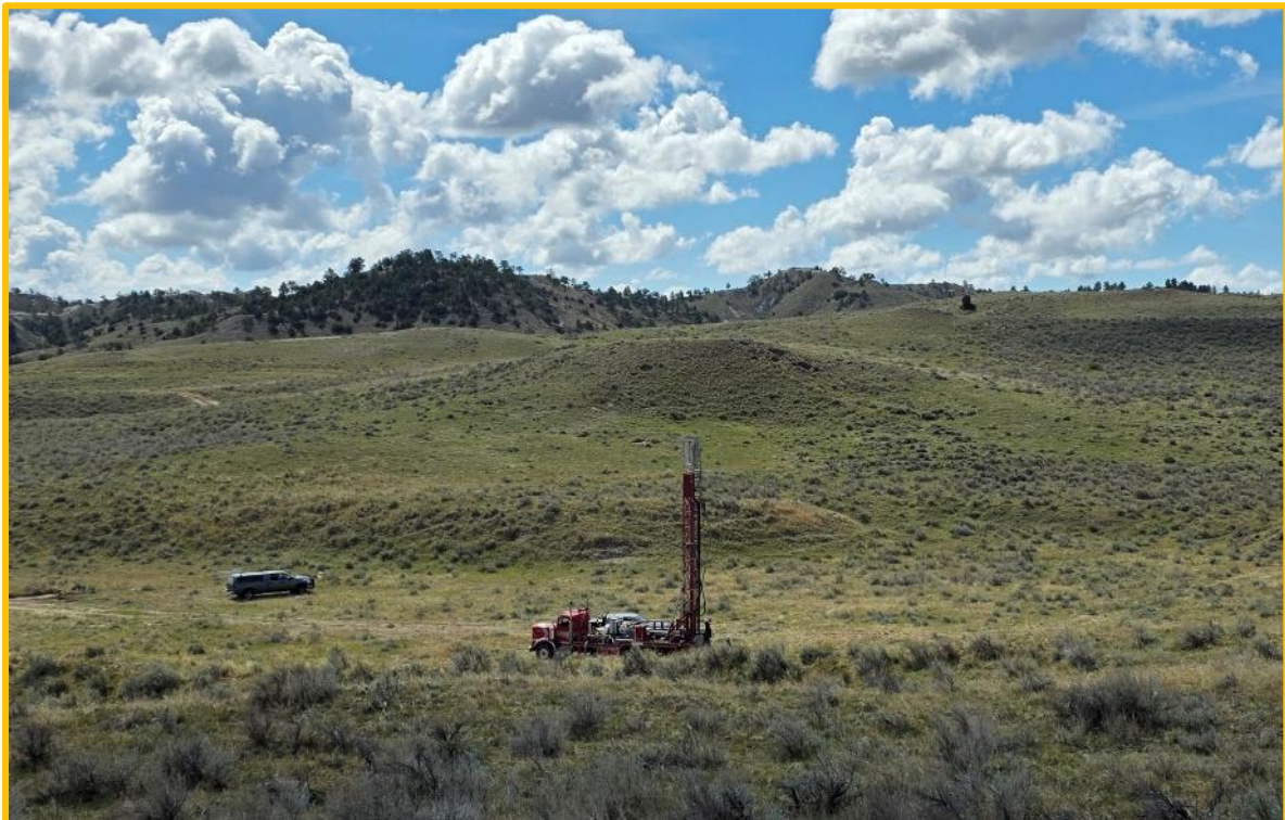
FIGURE 4: MUD ROTARY DRILL RIG AT MINE UNIT 1
