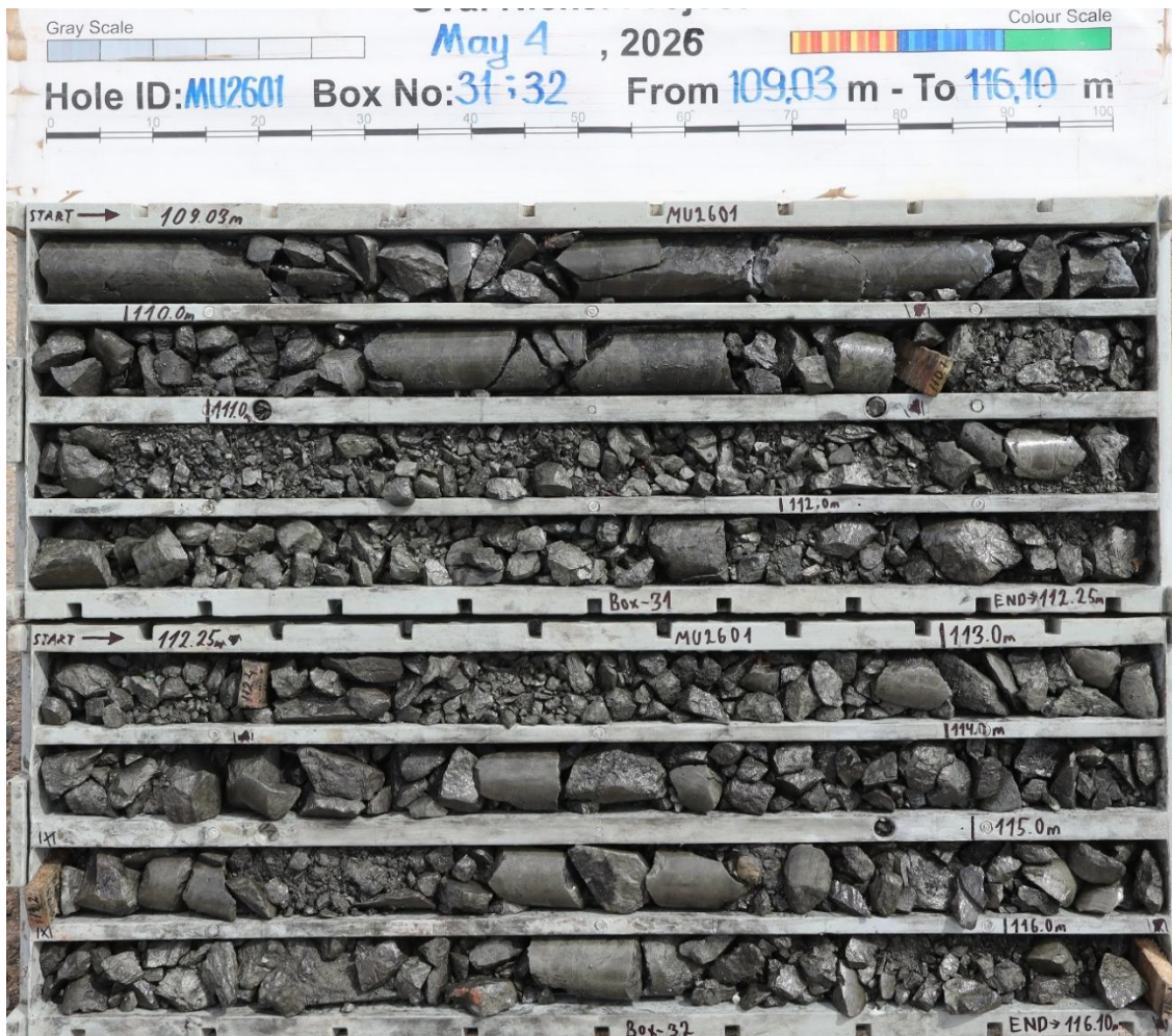
Photo 1. The massive sulphide mineralisation in drillhole MU2601. Parts of longer mineralised intervals included as an illustration of the nature of mineralisation. Mineral abbreviations are provided in Table 1
