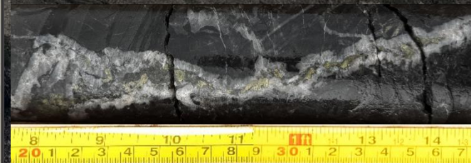
Example of chalcopyrite-bornite hosting quartz-carbonate veining within the lower Rae Group sediments of STK25001 between 1x81.30 and 181.52m downhole. Core diameter is NQ2.
